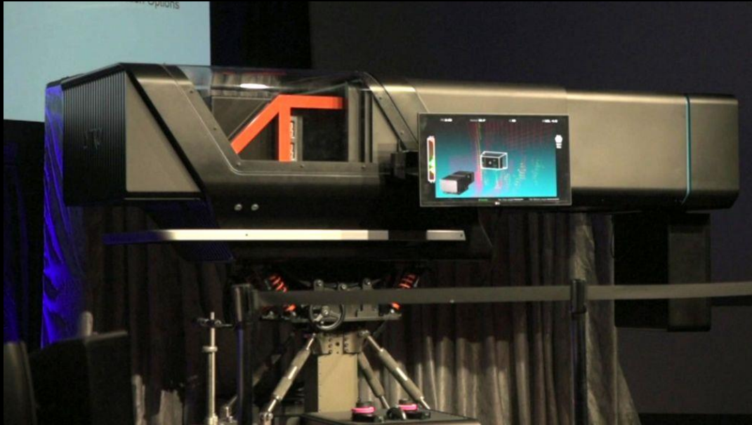
Lenslet-based light field imager 755 MPixel sensor
