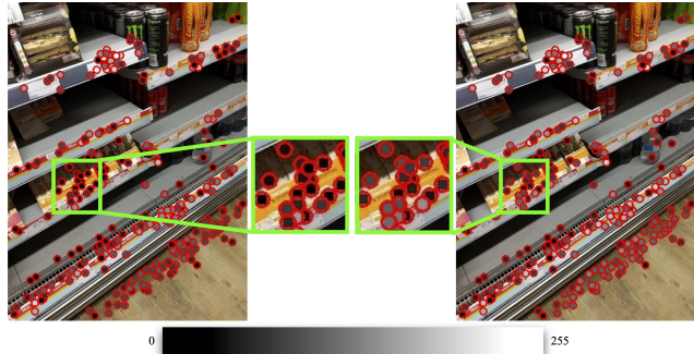
Figure 4. To illustrate the difference between our proposed time-infused score and the plain visibility score (i.e. the number of cameras a point was viewed from), we selected a random picture from the live map and project the map onto it. Each point here is associated with a stability score \sigma^i (left image) and a visibility score v_1 (right image). The higher the value, the more stable the point is. Most of the products’ points from the left cropped-image are darker from the ones in the right. This confirms our hypothesis, that those points on the products (i.e. dynamic objects) are less likely to be used for pose estimation using our score \sigma^i .
