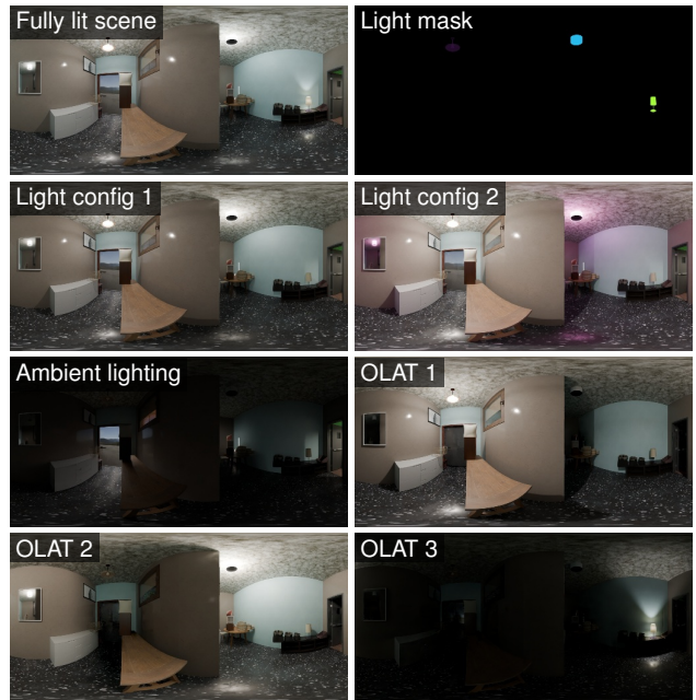
Figure 3. Synthetic multi-light data example. Our synthetic dataset comprises over 12,000 indoor scenes with procedurally generated light sources, each rendered as equirectangular images under multiple lighting conditions: fully lit, randomly lit, ambient only, and one-light-at-a-time (OLAT). During training, we sample perspective views from these equirectangular images on the fly.
