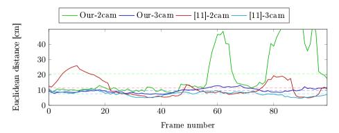
**Fig. 4.** Influence of the number of camera views. Using three cameras, our reconstruction is as accurate as tracking with the manual model. It is still accurate for two cameras for large parts of the sequence.
