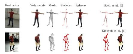
Fig. 1. Comparison of the estimated actor models for the Walk sequence (top) and Marker sequence (bottom) to the manually created skeletons of Stoll et al. [6] and Elhayek et al. [1]. For comparison between methods, we represent Gaussians as spheres with radius equal to one standard deviation.
